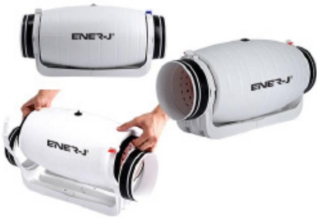
As the name suggests these fans are extremely quiet, low profile “Mixed-flow” fans. Manufactured in plastic material with an external connection box. The body is easily dismantled with full speed controllable, triple speed motor. Sounds waves are directed through the perforated inner skin and absorbed by a layer of sound-absorbent insulation. Plus the W- SILENT is fitted with rubber gaskets on the inlet and outlet to absorb vibrations
