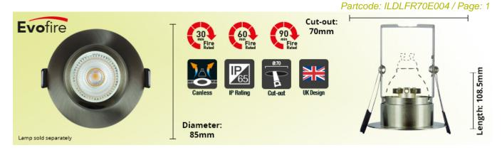
The Evofire Fire Rated Downlight is a safe and attractive fitting for a GU10 or MR16 LED lamp. The fully open design of the Evofire does not conceal your lamp in a large metal canister, which can trap some of the heat it generates, lowering lamp lifetime and performance. Lamps installed in an Evofire run at up to 10 degrees C cooler than a typical can-style fire rated downlight from leading LED brands - this can extend the lifetime of your lamps.
